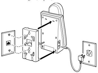
2. After charging, remove the twist-tie from the phone cord and plug the modular telephone connector into the
